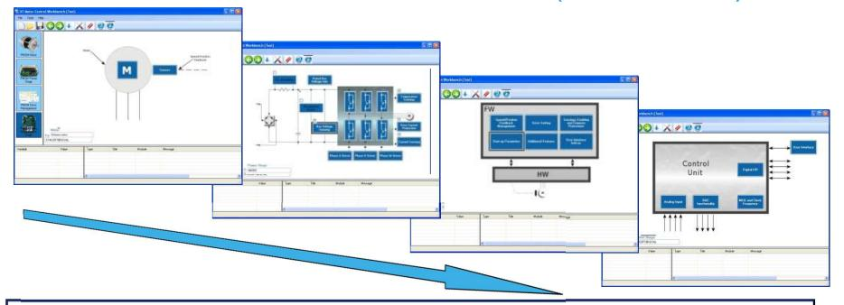
ST Motor Control Workbench, in this version, is a PC code generator tool that reduces the designer effort and time in the firmware development for all the ST Motor control FW library (starting from STM32 PMSM FOC FW library 3.0). The user through a graphical user interface (GUI) generate the parameter header files which configures the library according the application needs.
